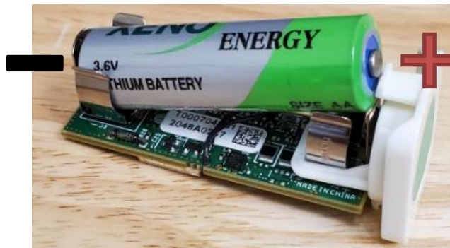
Figure 2-6: Battery Polarity Orientation
