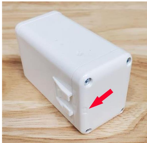
Figure 2-11: Proper Replacement Orientation of the Battery Cover
