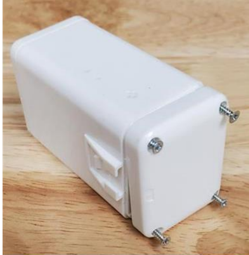
Figure 2-8: Removing the Battery Cover Screws
