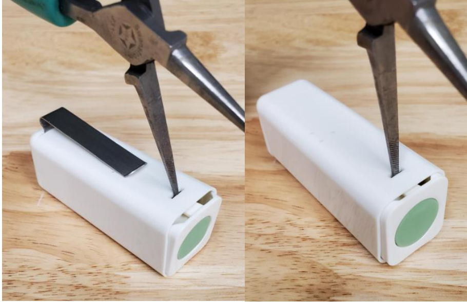
Figure 2-5: Using a Tool to Release the End-Cap
